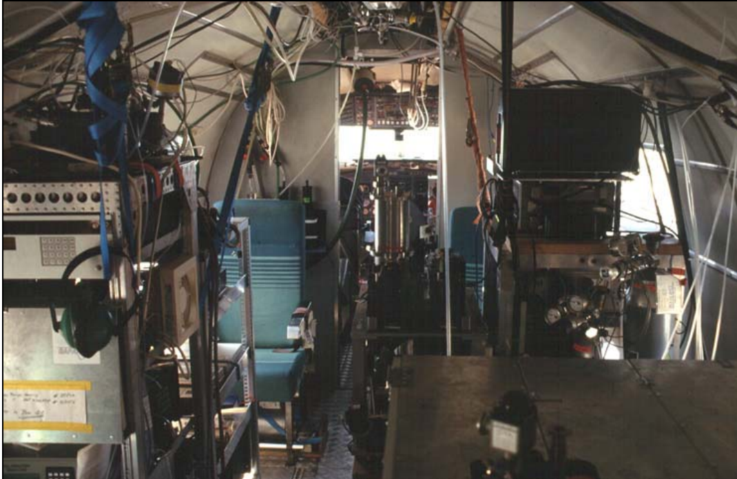
Figure 4. DC-3 research aircraft of the Max Planck Institute for Chemistry used for aerial VFS measurements during the SAFARI-92 campaign. Source: GFMC
