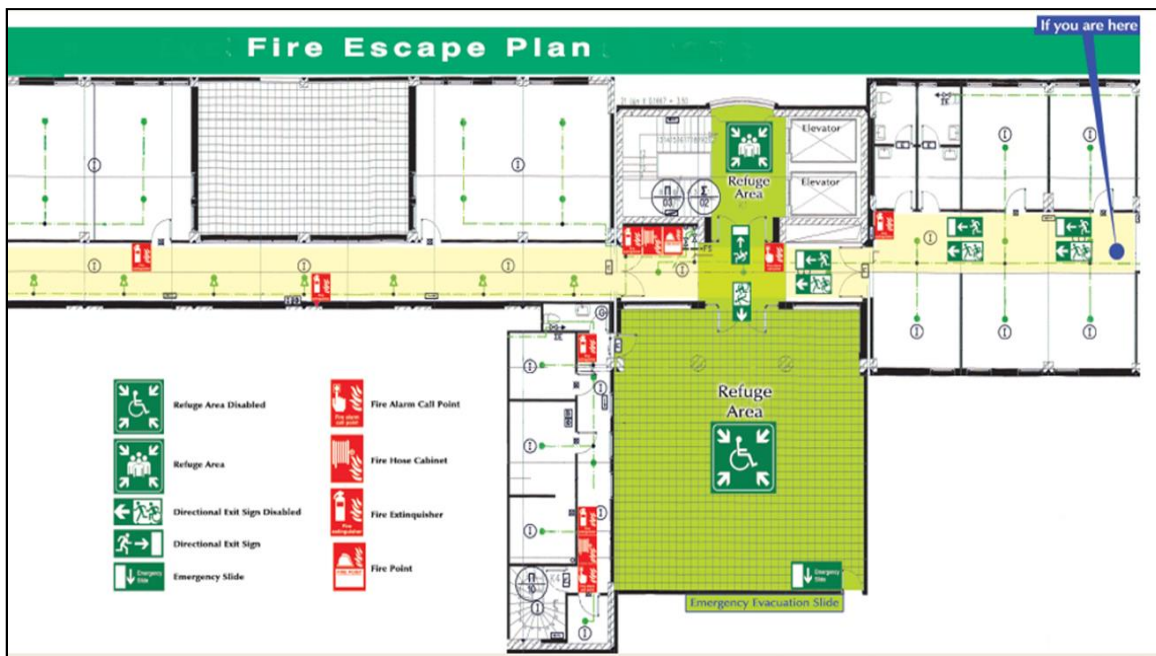
Indicative example of a building’s “Fire Escape Plan” according to ISO 23601:2020, including accessible means of egress icon (European Center for Forest Fire, “Evacuation Planning of Critical Infrastructures in case of an Earthquake or a Fire for People with Disabilities, 2016”)
